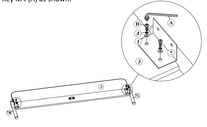
STEP 3: Attach (6) to (4) and (5) With (D),(J) and (I) Using a Allen Key M4 (A) as shown.
