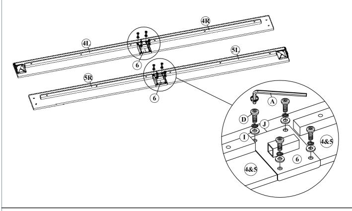
STEP 4: Attach Assembled (3) to (4) and (5) With (D),(J) and (I) Using a Allen Key M4 (A) as shown.
