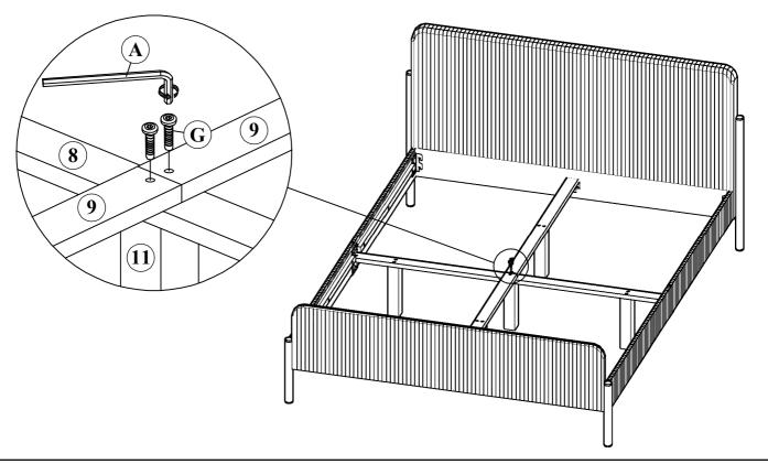
STEP 10: Attach Assembled Bed Slats to Assembled Bed Frame with (H) Using a Allen Key M4 (A) as shown.
