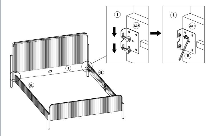
STEP 6: Attach Assembled Bed Slats to Assembled Bed Frame with (C) Using a Allen Key M4 (A) as shown.
