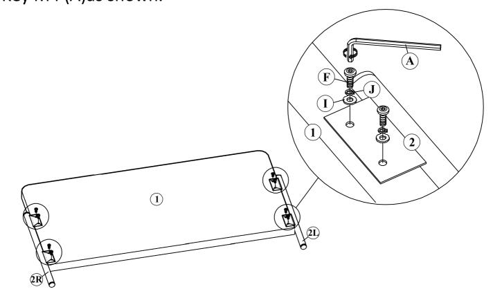
STEP 2: Attach the (7) to (3) by using (D),(J) and (I) with Allen Key M4 (A) as shown.
