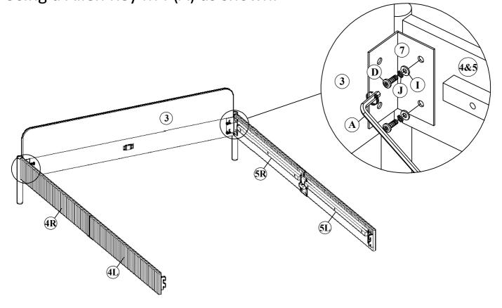
STEP 5: Attach (4) and (5) to Assembled Headbaord as shown.
